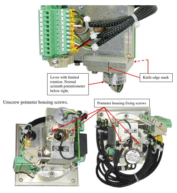
Unscrew potmeter fixing screws and pull out potmeter unit. Loosen clamping ring from potmeter axle. Replace the potmeter. Reassemble the unit, slide it into the lever and fix it with two screws and washers, after adjusting potmeter roughly. Reconnect the potmeter wires.
