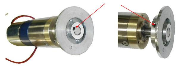
Adjust motor against the clutch, as close as possible without touching it.
