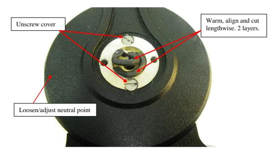
A sleeve is used to splice these two wires. The sleeve is removed by squeezing it open. Pull gently off. If this is not possible it can be cut off, but make sure the wires are long enough to be joined later.
