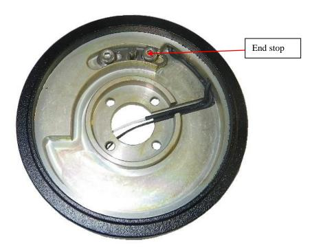
Note end stop position before dismounting it. (To avoid later adjustment) Install the new end stop in the same location as the old.
