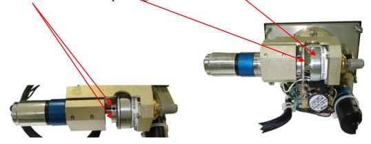
Pull motor out of motor bracket.
