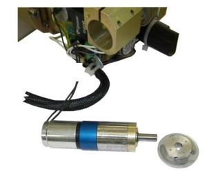
Push a new motor into the bracket, and thread magnet disc on the motor axle.
