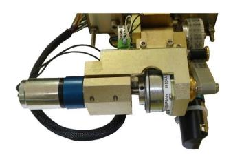
Disconnect motor wires. Loosen bracket screws to loosen motor.
