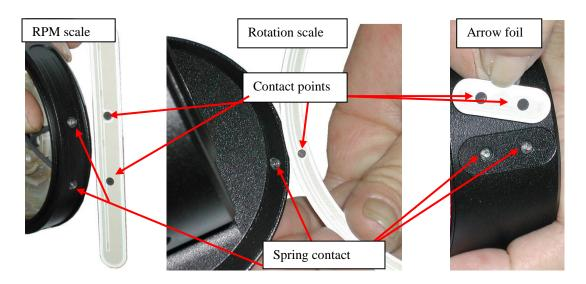
Then fasten the scale to the lever with high pressure from your finger. Press out air bubbles. When changing the rotation scale, be assure to place the zero point on the white reading point of the panel plate.
