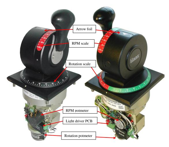
Remove old scale. Be aware the small plastic tube/ring placed between the contact spring and its metal surroundings. It may follow the old scale and must be replaced.
