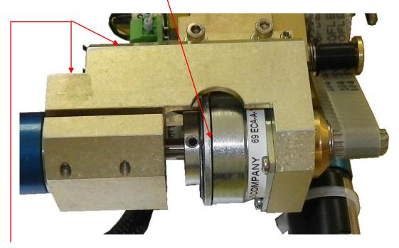
Tighten fixing screws on the motor bracket. Connect wires.
