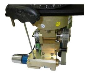
Uncsrew 2 set screws to split magnet disc from the clutch.
