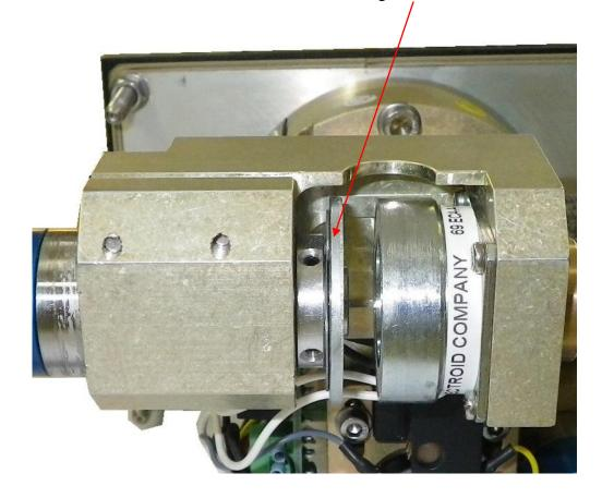
Important: To fix set screws, the notch in the disc must align with the flat area on the axle. Axle and disc position is illustrated below. The axle must not penetrate the disc completely.
