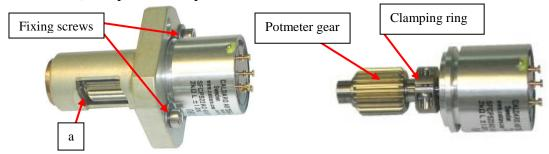
Loosen screws on potmeter gear and clamping ring and replace the potmeter with the new one. Adjust gear position by moving the clamping ring on the potmeter axle. The gear must move freely, se the space market a above. Fix potmeter in housing with two fixing screws and washers after adjusting potmeter roughly.
